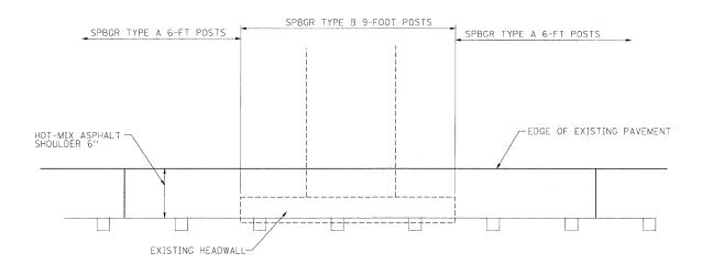
NOTE: LENGTH OF SHOULDER WIDENING TO BE DETERMINED BY ENGINEER
