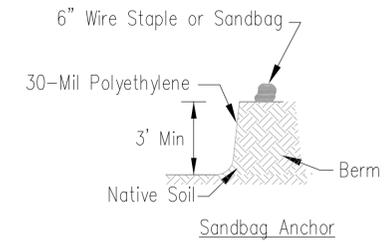
EARTHEN BERM ANCHOR SECTIONS
