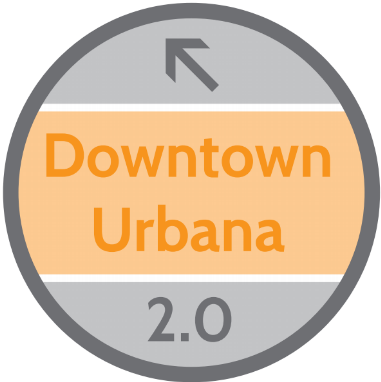
Sample LARGE ENTRANCE SIGN, Colorcore Sign, Circular, 20" Diameter Note: Sign colors shown on this page are for example only. Actual colors are shown on the plans.
