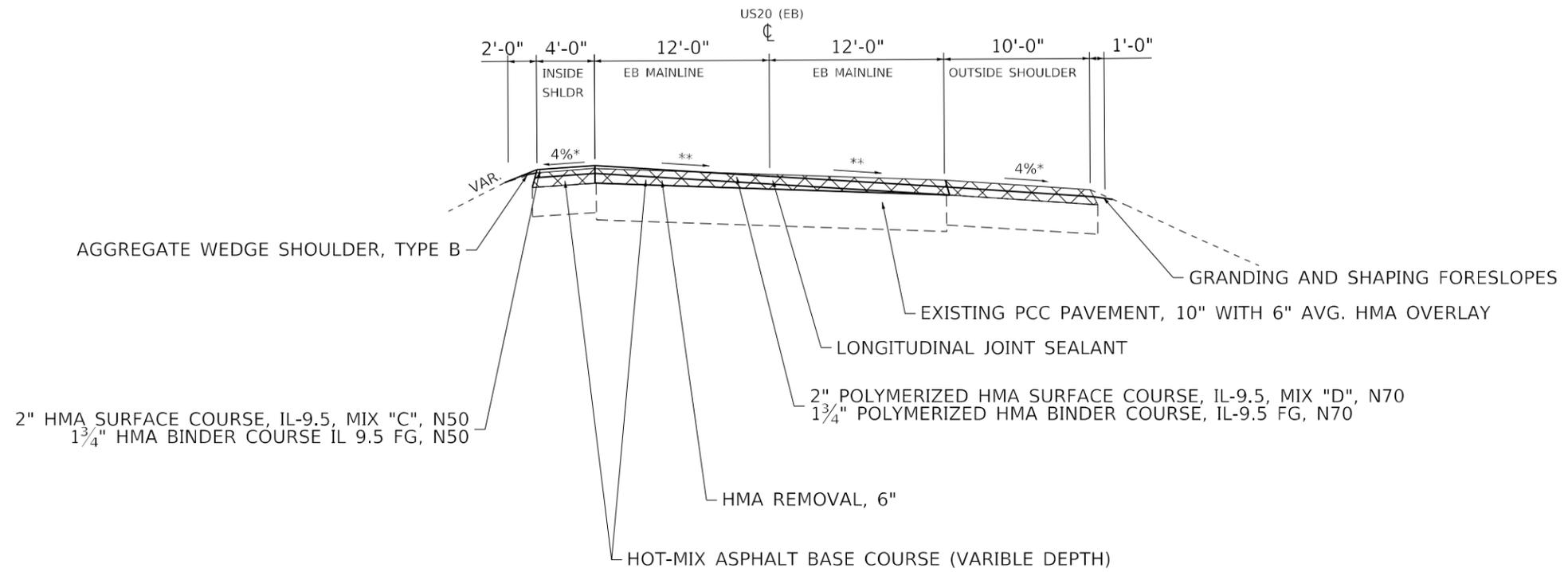
\* OUTSIDE EDGE SHALL MAINTAIN A MAX OF 8% OF SUPERELEVATION WITH RESPECT TO THE PAVEMENT.
