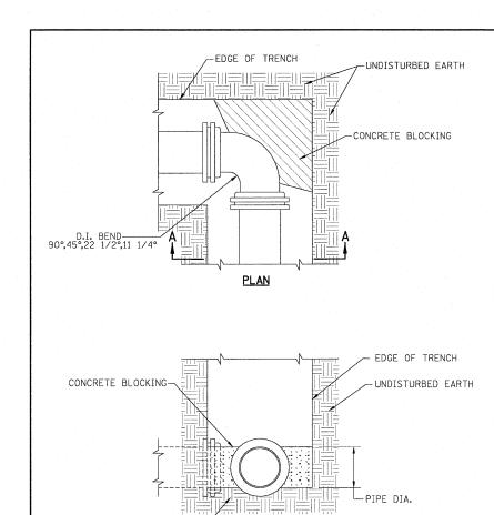
UNDISTURBED EARTH-SECTION A-A (BEDDING SHALL BE PROVIDED AS REQUIRED BY CONTRACT PLANS AND D.I. BENDS SPECIFICATIONS)
