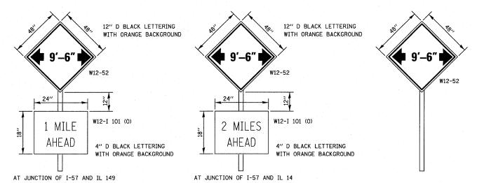
A W12-52 SIGN. WITH A W12-I101 SIGN, SHALL BE ERECTED AT THE JUNCTION OF I-57 AND IL 149 AND AT THE JUNCTION OF I-57 AND IL 14. THE ACTUAL LOCATION OF THE SIGNS TO BE DETERMINED BY THE ENGINEER. AN ADDITIONAL W12-52 SIGN SHALL BE ERECTED 1000 FEET IN EACH DIRECTION FROM THE INTERCHANGE PRIOR TO STAGE 1 CONSTRUCTION. THESE SIGNS SHALL BE MAINTAINED BY THE CONTRACTOR DURING STAGE CONSTRUCTION AND SHALL BE REMOVED AT THE COMPLETION OF ALL STAGED CONSTRUCTION.
