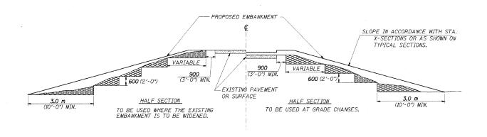
MATERIAL TO BE REMOVED AND REPLACED IN THE EMBANKMENT IN ACCORDANCE WITH ART. 205.04 OF THE STANDARD SPECIFICATION. COST TO BE INCLUDED IN THE VARIOUS ITEMS OF EXCAVATION AND NO ADDITIONAL COMPENSATION WILL BE ALLOWED BECAUSE OF THIS WORK.
