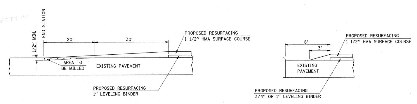
BUTT JOINT 40TH. ST. LOCATIONS 0+00, 15+25 (FROM SOUTH) EDGE OF PAVEMENT SURFACE COURSE TAPER
