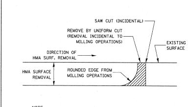
WHEN MILLING OPERATIONS PRODUCE A ROUNDED EDGE, THEN A SAW CUT SHALL BE USED TO MANUFACTURE A PERPENDICULAR EDGE AS SHOWN IN THE DETAIL. THE ENGINEER SHALL BE THE SOLE JUDGE CONCERNING THE USE OF THIS DETAIL
