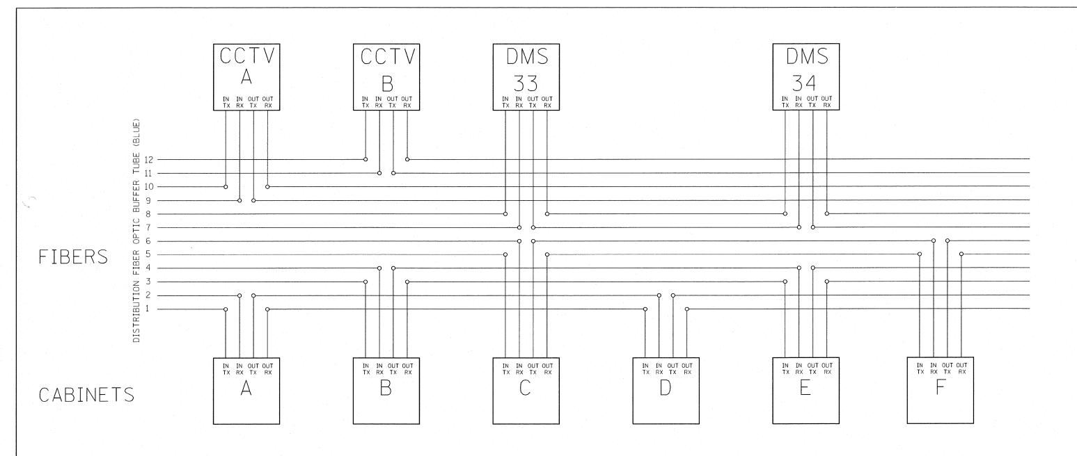
FIBERS 1 AND 2 CABINETS 1, 4, 7, 10, 13, 16, 19, 22, 25, 28, 31, 34, 37, 40, 43, 46, 49. FIBERS 3 AND 4 CABINETS 2, 5, 8, 11, 14, 17, 20, 23, 26, 29, 32, 35, 38, 41, 44, 47, 50. FIBERS 5 AND 6 CABINETS 3, 6, 9, 12, 15, 18, 21, 24, 27, 30, 33, 36, 39, 42, 45, 48. FIBERS 7 AND 8 DMS 33, DMS 34. FIBERS 9 AND 10 CCTV 50, 49, 47B, 47, 45, 43A, 42, 40, 38, 37, 35A, 34, 32, 30A, 29. FIBERS 11 AND 12 CCTV 51, 49A, 48, 47A, 46, 44, 43, 40A, 39, 37A, 36, 35, 32A, 31, 30.
