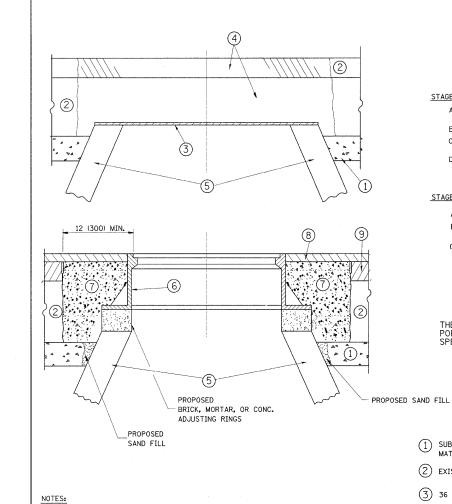
EXISTING BROKEN FRAMES AND LIDS SHALL BE REMOVED AND DISPOSED OF BY THE CONTRACTOR AND SHALL BE REPLACED AS DIRECTED BY THE ENGINEER. REPLACEMENT FRAMES AND LIDS WILL BE PAID FOR IN ACCORDANCE WITH ARTICLE 109.04 OF THE STANDARD SPECIFICATIONS
