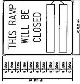
THESE SIGNS ARE REQUIRED ON BOTH SIDES OF THE RAMP, MINIMUM OF 1 WEEK IN ADVANCE OF THE CLOSURE.
