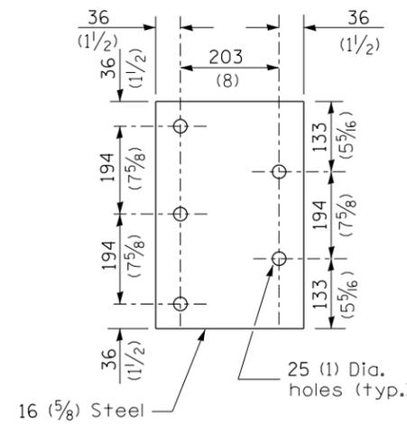
PARAPET STEEL BEARING PLATE DETAIL
