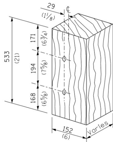
MODIFIED THICKNESS WOOD BLOCKOUT DETAIL
