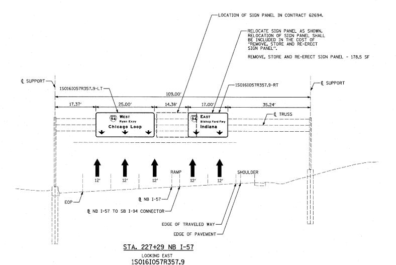
NOTE: EXISTING SIGN STRUCTURE AND SIGN PANELS WERE INSTALLED DURING CONTRACT 62694. THE SIGN AT THE RIGHT WAS PLACED IN A LOCATION TO AGREE WITH THE ROADWAY CONDITIONS AT THE END OF CONTRACT 62694. DATA USED TO CONSTRUCT THE OVERHEAD SIGN STRUCTURE IS INCLUDED IN THE PLANS FOR INFORMATION ONLY.
