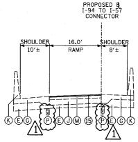
PROPOSED WB I-94 TO I-57 CONNECTOR STA. 314+60 TO RECONSTRUCTION LIMIT
