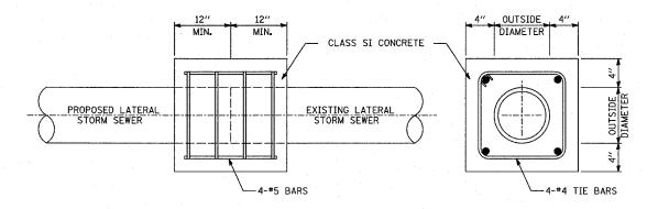
THE PROPOSED CONCRETE COLLAR SHALL OVERLAP EACH STORM SEWER PIPE A MINIMUM OF 1 FOOT.
