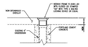
PROPOSED IN-PAVEMENT **UNDERDRAIN INSPECTION** HOLE ADJUSTMENT
