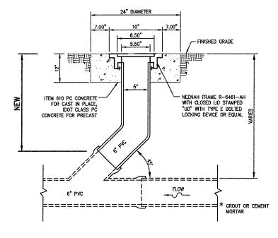
PROPOSED UNDERDRAIN **CLEANOUT ADJUSTMENT**
