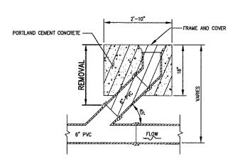
**EXISTING UNDERDRAIN** CLEANOUT REMOVAL
