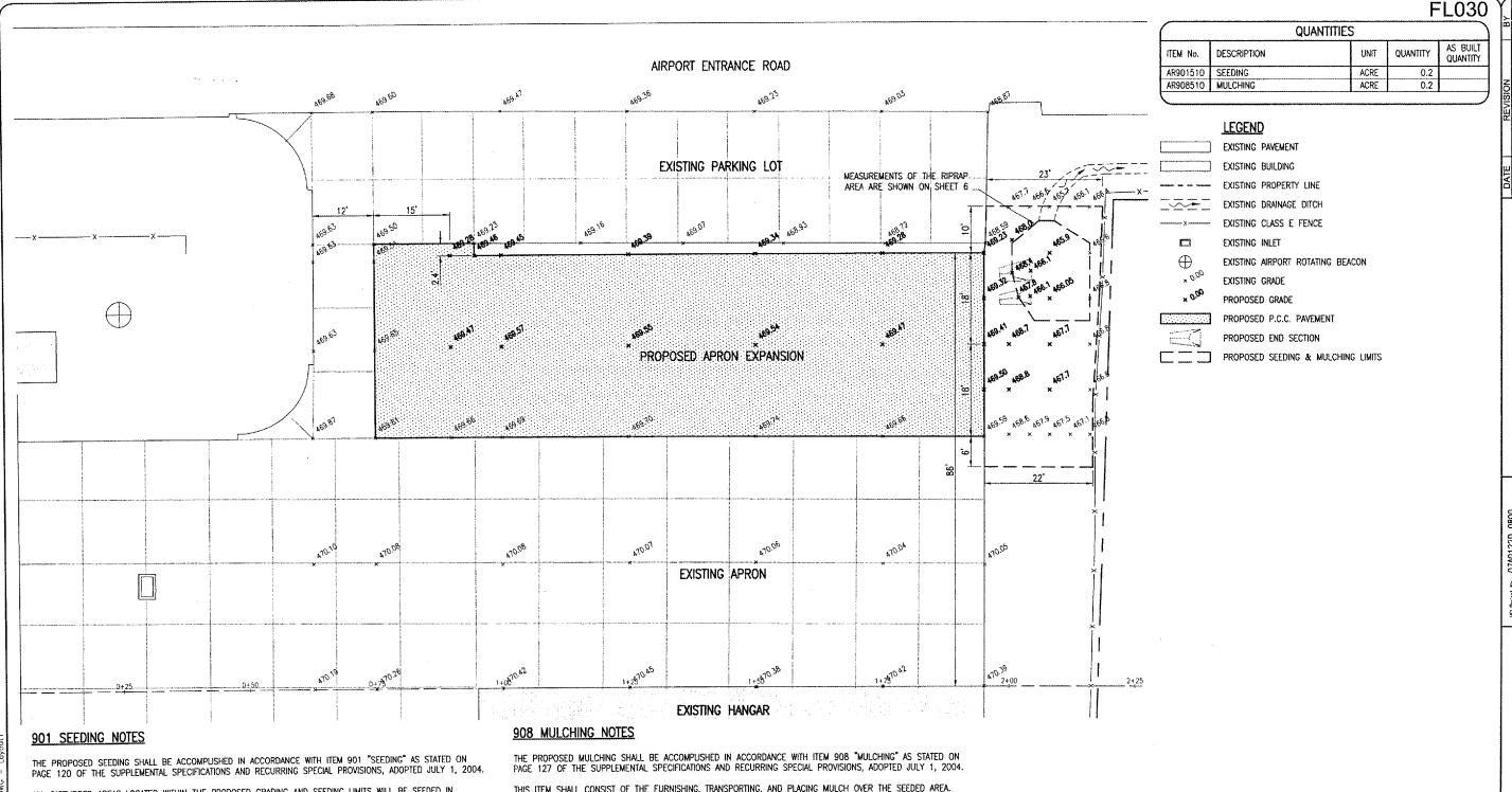
ALL DISTURBED AREAS LOCATED WITHIN THE PROPOSED GRADING AND SEEDING LIMITS WILL BE SEEDED IN ACCORDANCE WITH THE ABOVE NOTED SPECIFICATION. ALL AREAS OUTSIDE THE DESIGNATED GRADING AND SEEDING LIMITS WILL ALSO BE SEEDED BUT AT THE CONTRACTOR'S OWN EXPENSE.
