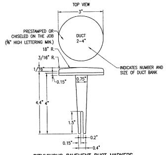
BITUMINOUS PAVEMENT DUCT MARKERS "NOT TO SCALE"
