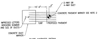
DUCT MARKER DETAIL "NOT TO SCALE"
