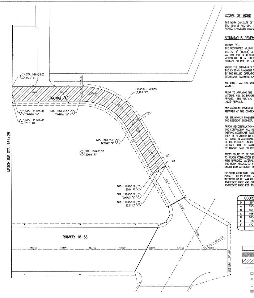
THE WORK CONSISTS OF THE RECONSTRUCTION OF TAXIWAY "A" BETWEEN STA. 150+95 AND STA. 170+54. THE WORK INCLUDES MILLING, ASPHALT PAVING, SHOULDER ADJUSTMENT, SEEDING AND TAXIWAY MARKING.
