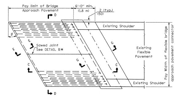
BRIDGE APPROACH PAVEMENT CONNECTOR (FLEXIBLE)
