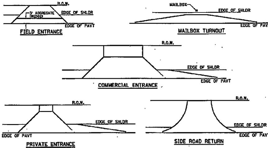
**NOTE:** EXISTING HMA PE's, CE's, SR's, & MB TURNOUTS
