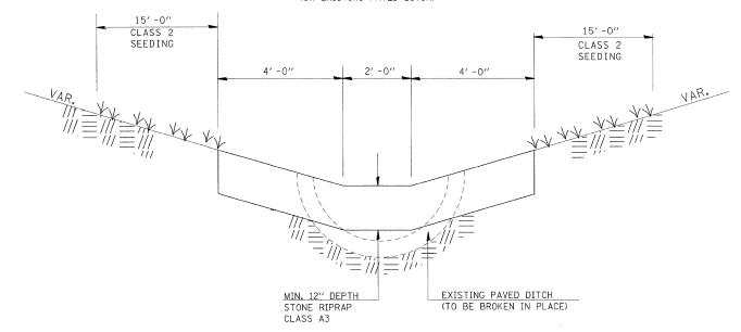
NOTES: THIS WORK SHALL BE PAID FOR AT THE CONTRACT UNIT PRICE PER TON, FOR STONE RIPRAP DITCH, WHICH PRICE SHALL INCLUDE ALL MATERIAL LABOR AND EQUIPMENT TO COMPLETE THE WORK IN PLACE AS SHOWN AND DETAILED IN THE SPECIAL PROVISIONS.
