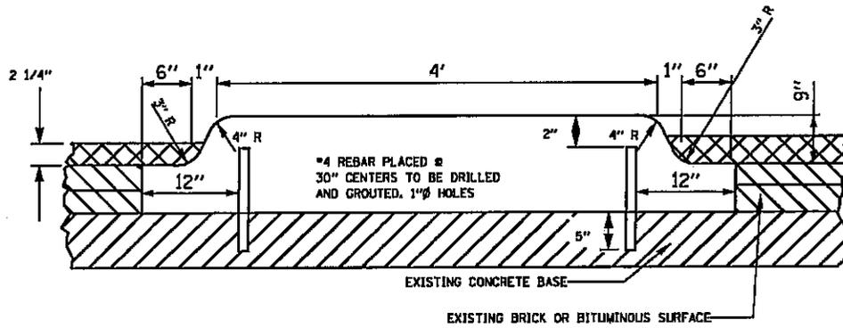
DETAIL OF CONCRETE MEDIAN, TYPE SB, SPECIAL
