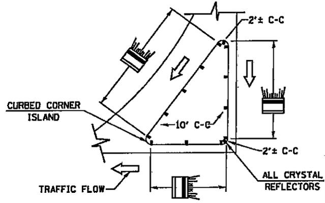
TYPICAL PLACEMENT OF PRISMATIC REFLECTORS ON CURBS
