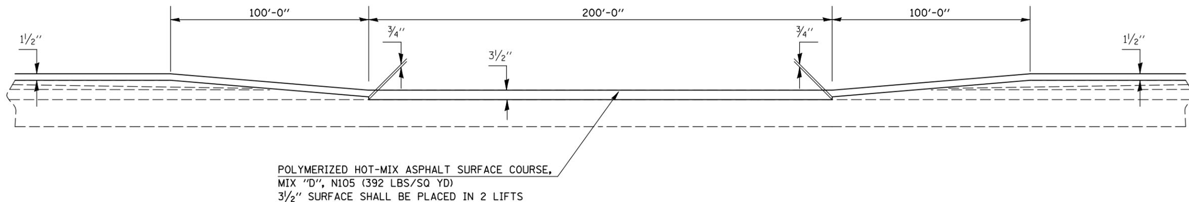
POLYMERIZED HOT-MIX ASPHALT SURFACE COURSE, MIX "D", N105 (392 LBS/SQ YD)
