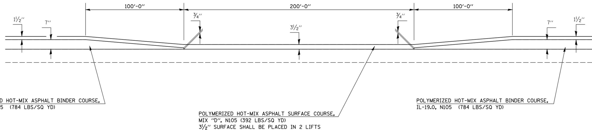
POLYMERIZED HOT-MIX ASPHALT BINDER COURSE, IL-19.0, N105 (784 LBS/SQ YD)
