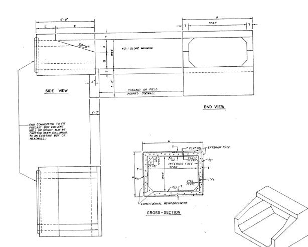
DETAIL OF PRECAST CONCRETE BOX CULVERT END SECTION
