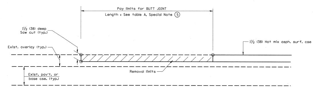
CASE 5: WITH HOT MIX ASPHALT SURFACE REMOVAL (COLD MILLING)
