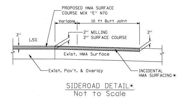
\* HMA SURFACE COURSE MIX "E" N70 TO REPLACE INCIDENTAL HMA SURFACE MIX AT IL 98, SHERIDAN, AND WILLOW AND EIGHTH INTERSECTIONS.
