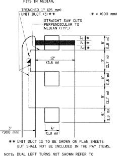
PLAN SHEET FOR DETECTOR LOOP REPLACEMENT
