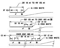
\* TURN LAMES IN EXCESS OF 400' (120 m) IN LENGTH MAY HAVE AN ADDITIONAL SET OF ARROW - "ONLY" INSTALLED MIDWAY BETWEEN THE OTHER TWO SETS OF ARROW - "ONLY".
