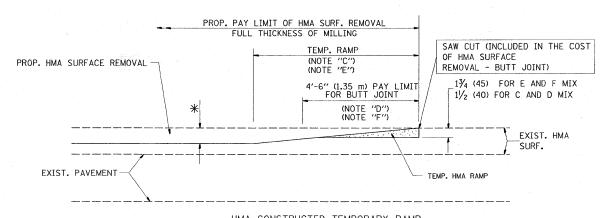
HMA CONSTRUCTED TEMPORARY RAMP (FOR BUTT JOINT AND HMA TAPER SEE DETAIL BELOW)
