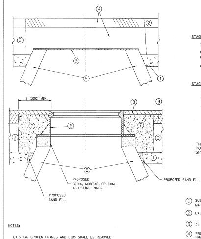
EXISTING BROKEN FRAMES AND LIDS SHALL BE REMOVED AND DISPOSED OF BY THE CONTRACTOR AND SHALL BE REPLACED AS DIRECTED BY THE ENGINEER. REPLACEMENT FRAMES AND LIDS WILL BE PAID FOR IN ACCORDANCE WITH ARTICLE 109,04 OF THE STANDARD SPECIFICATIONS UNLESS A SEPARATE PAY ITEM HAS BEEN PROVIDED.
