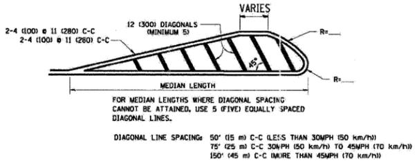
DIAGONAL LINE SPACING: 50' (15 m) C-C (LESS THAN 30MPH (50 km/h))
