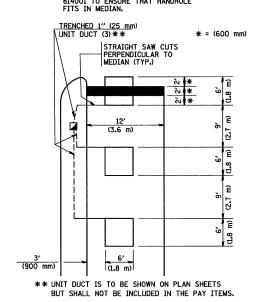
PLAN SHEET FOR DETECTOR LOOP REPLACEMENT
