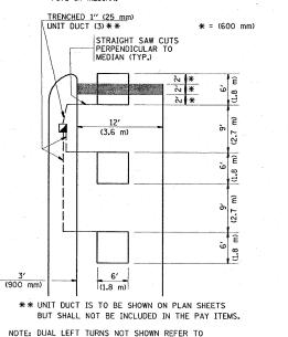
PLAN SHEET FOR DETECTOR LOOP REPLACEMENT
