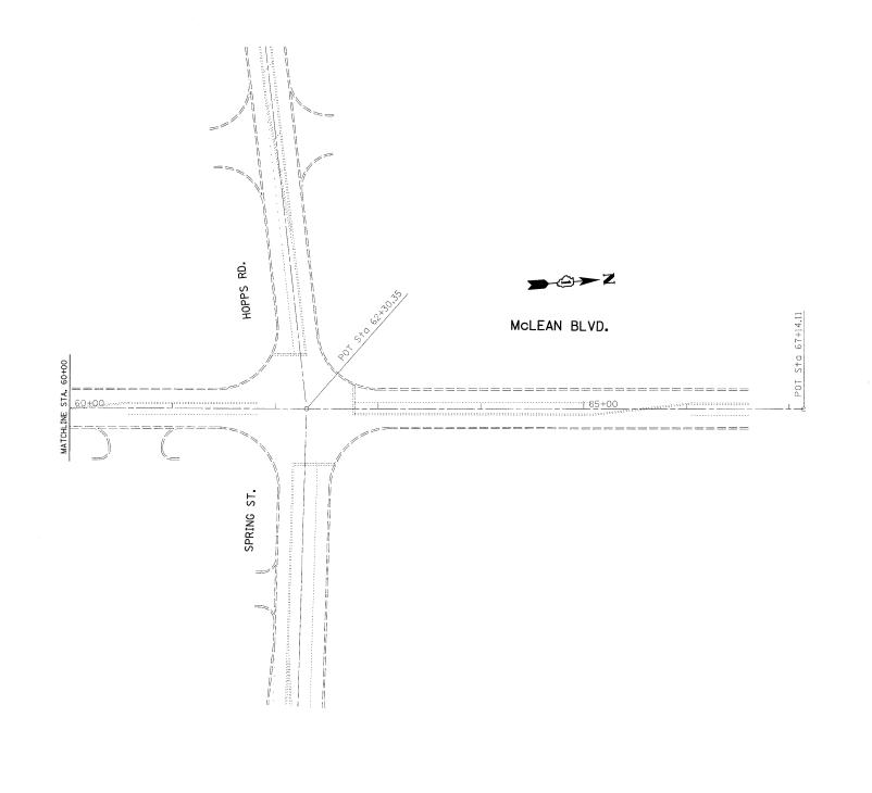
NOTE LIMIT OF RESURFACING ON SIDE-STREETS THROUGH OUT THE IMPROVEMENT SHALL BE TO THE RADIUS OF RETURN OR AS DIRECTED BY THE ENGINEER.
