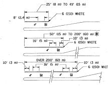
FULL SIZE LETTERS 8' (2.4 m) AND ARROWS SHALL BE USED.  $\P$  AREA = 15.6 SO. FT. (1.5 m<sup>2</sup>) MV AREA = 20.8 SO. FT. (1.9 m<sup>2</sup>)
