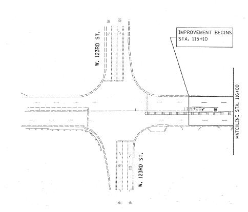
NOTES: LIMIT OF RESURFACING ON SIDE-STREETS THROUGH OUT THE IMPROVEMENT SHALL BE TO THE RADIUS OF RETURN OR AS DIRECTED BY THE ENGINEER.
