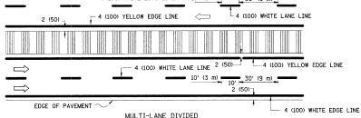
WITH MOUNTABLE MEDIAN NOTE: MEDIANS WITH BARRIER CURB DO NOT REQUIRE AN EDGE LINE
