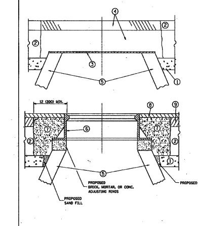
EXISTING BROKEN FRAMES AND LIDS SHALL BE REMOVED AND DISPOSED OF BY THE CONTRACTOR AND SHALL BE REPLACED AS DIRECTED BY THE ENGINEER. REPLACEMENT FRAMES AND LIDS WILL BE PAID FOR IN ACCORDANCE WITH ARTICLE 109.40 OF THE STAMDARD SPECIFICATIONS UNLESS A SEPARATE PAY ITEM HAS BEEN PROVIDED.
