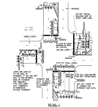
ARTERIAL-VOLUME DENSITY ("FAR OUT" DETECTION) CROSS STREET-NON VOLUME DENSITY ("UPTIGHT" PRESENCE DETECTION)
