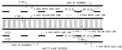
WITH MOUNTABLE MEDIAN NOTE: MEDIANS WITH BARRIER CURB DO NOT REQUIRE AN EDGE LINE
