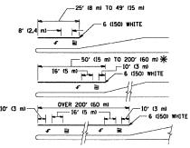
\*\* TURN LAMES IN EXCESS OF 400' (120 m) IN LENGTH MAY HAVE AN ADDITIONAL SET OF ARROW - "ONLY" INSTALLED WIDWAY BETWEEN THE OTHER TWO SETS OF ARROW - "ONLY".
