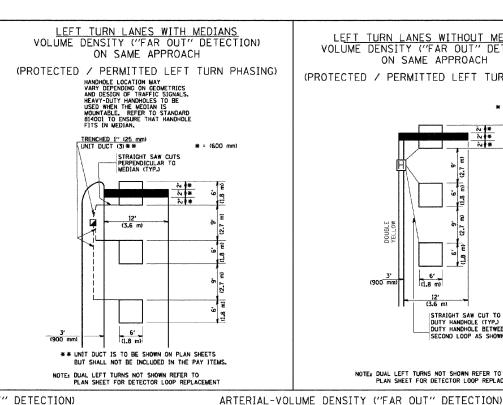
VOLUME DENSITY ("FAR OUT" DETECTION) ON SAME APPROACH (PROTECTED / PERMITTED LEFT TURN PHASING) # = (600 mm) (1.8 m) (900 mm) 12' (3.6 m) STRAIGHT SAW CUT TO HEAVY DUTY HANDHOLE (TYP.) PLACE HEAVY DUTY HANDHOLE BETWEEN FIRST AND NOTE: DUAL LEFT TURNS NOT SHOWN REFER TO PLAN SHEET FOR DETECTOR LOOP REPLACEMENT
