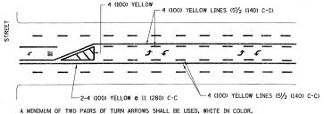
A MINIMUM OF TWO PAIRS OF TURN ARROWS SHALL BE USED, WHITE IN COLOR. DDITIONAL PAIRS SHALL BE PLACED AT 200' (60 m) TO 300' (90 m) INTERVAL
