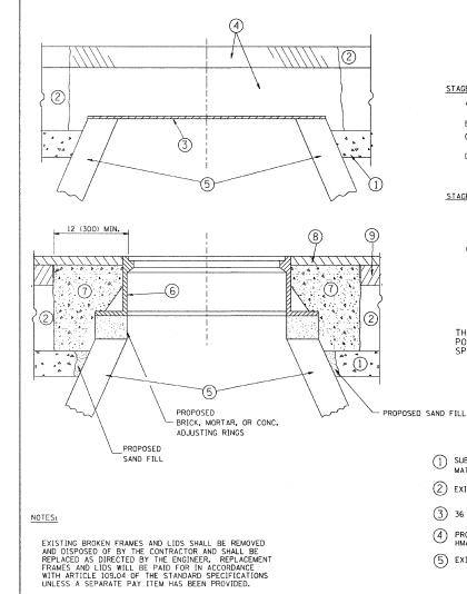
IF THE EXISTING LIDS ARE OPEN, THE FRAME WILL BE ADJUSTED TO THE ELEVATION OF THE MILLED PAVEMENT SURFACE PRIOR TO THE MILLING OPERATION. THE FRAME WILL NOT BE REMOVED AND COVERED BY THE METAL PLATE.
