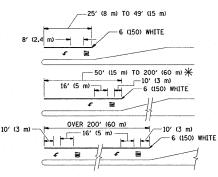
\* TURN LANES IN EXCESS OF 400' (120 m) IN LENGTH MAY HAVE AN ADDITIONAL SET OF ARROW - "ONLY" INSTALLED MIDWAY BETWEEN THE OTHER TWO SETS OF ARROW - "ONLY".
