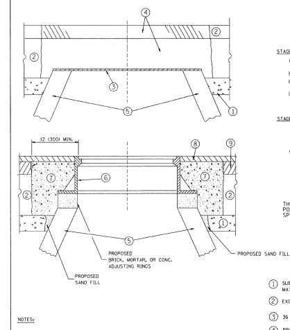
EXISTING BROKEN FRAMES AND LIDS SHALL BE REMOVED AND DISPOSED OF BY THE CONTRACTOR AND SHALL BE REPLACED AS DIRECTED BY THE REGINEER, REPLACEMENT FRAMES AND LIDS WILL BE PAID FOR IN ACCORDANCE WITH ARTICLE 109,04 OF THE STANDARD SPECIFICATIONS UNLESS A SEPARATE PAY ITEM HAS BEEN PROVIDED.
