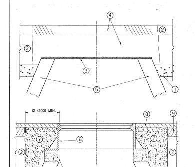
BRICK, MORTAR, OR CONC. ADJUSTING RINGS
